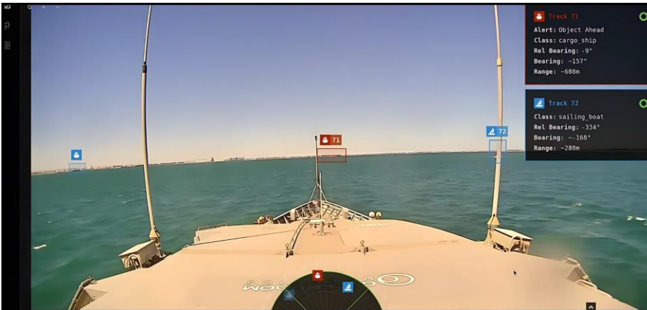
A sensor agnostic passive optical radar.
